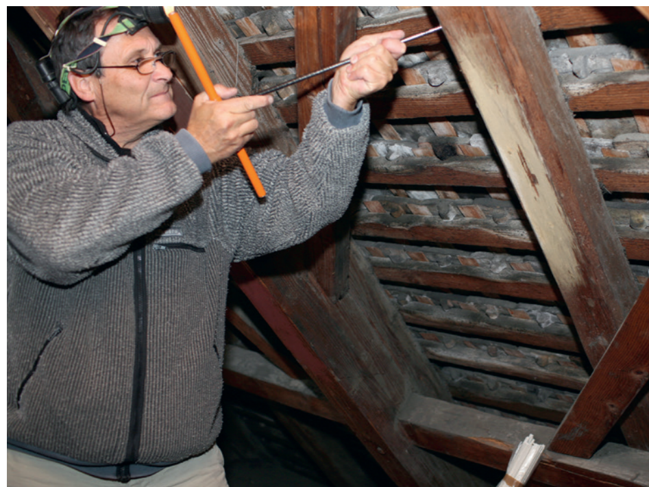
Sampling for dendrochronological analysis of roof truss.
