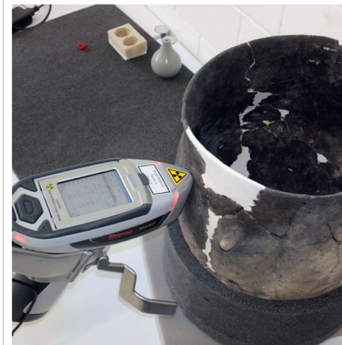
Material analysis of Neolithic ceramics using a portable X-ray fluorescence analysis device owned by the University of Berne. The aim is to distinguish between locally produced vessels and imitations.
